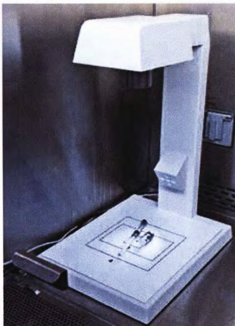
Figure 1. Inspection camera within the biological safety cabinet.
