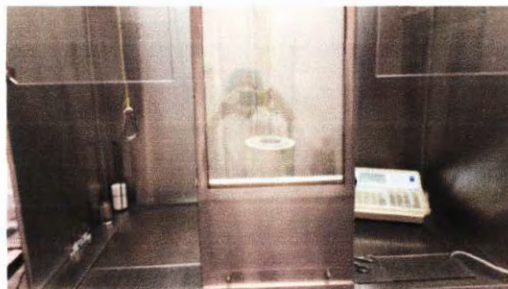
L-block lead glass shield and dose calibrator used inside of a LFH
