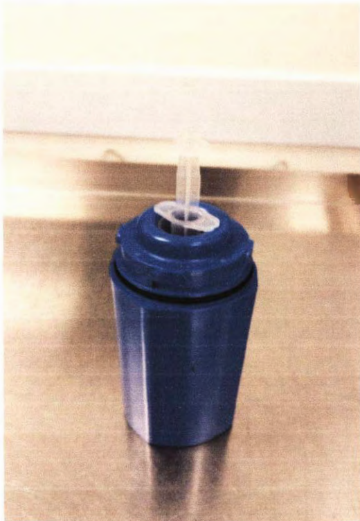
A "pig" used to transport doses to nuclear medicine clinics and departments for use in patients.
